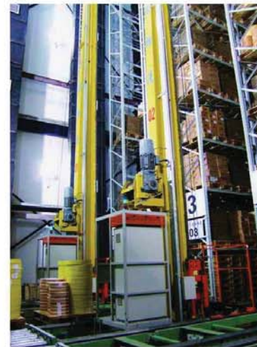
■ Aisle stacker crane for automatic retrieval and storage in high-bay warehouse
